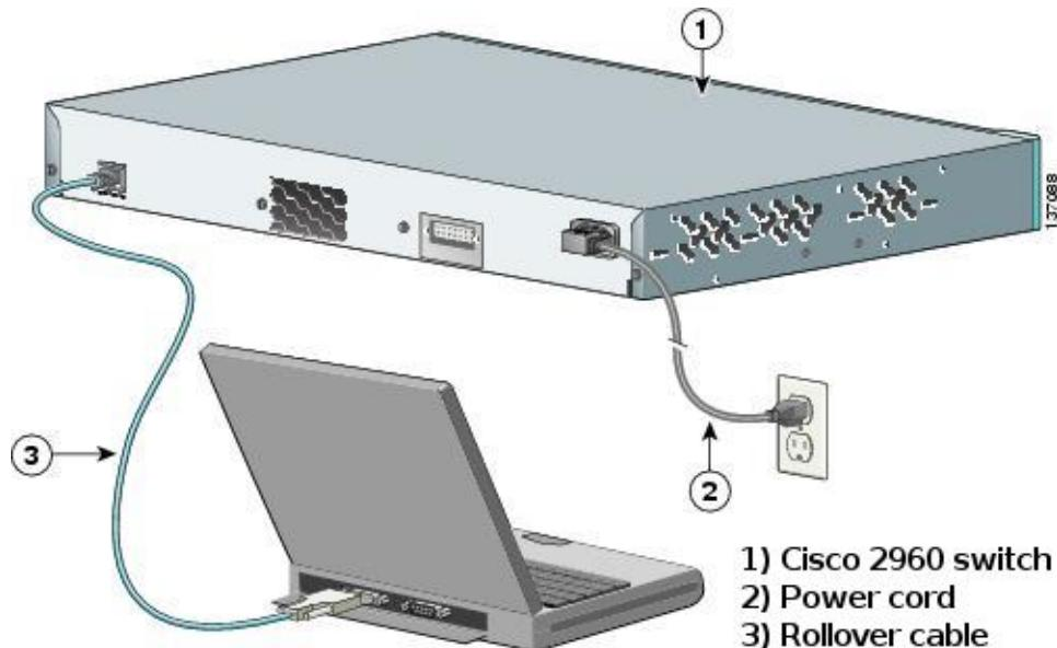
**Note:** Serial COM ports are no longer available on most computers. A USB-to-DB9 adapter can be used with the rollover console cable for console connection between the computer and a Cisco device. USB-to-DB9 adapters can be purchased at any computer electronics retailer.
